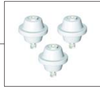
M8 Set of 3 Ø89 x 76 Polyfibre Base Insulators supplied with M7 pedestal base with 3 x 15mm slots on 200mm - 254mm PCD
